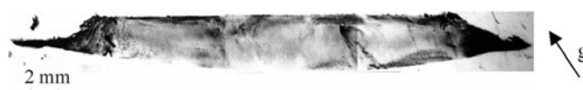
Figure 5. A vertical section (D-geometry) of a 4H-SiC ingot showing the enlargement of the crystal during the growth. The seed is at the upper level.
